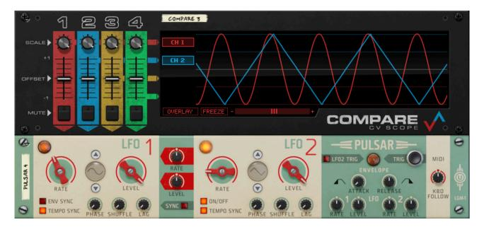
Now tweak the controls on Compare's channel 1 and 2 to the left on the front panel, and select different views using the view button in the lower left corner of the display.
