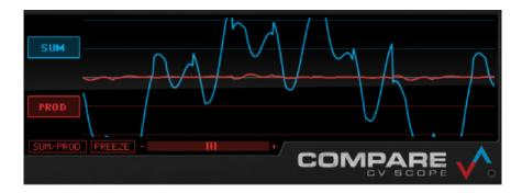
Multiplying the signals is the same as having the signals scale each other, like on a VCA in a synthesizer. Note that when you have a lot of periodic signals centered around 0, the Product will usually stay close to 0.
