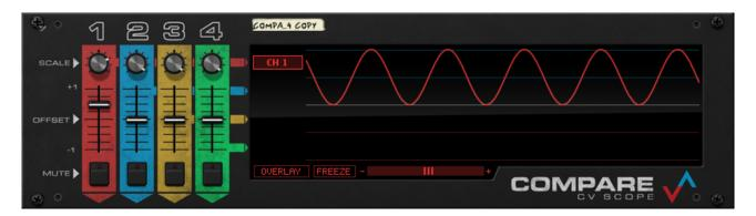
In the above image, our original sine curve has been scaled down by 50% and offset by +0.5 V.
