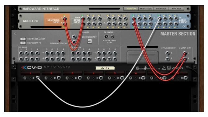
This setup will convert the LFO CV signal to audio, and send it to the output of your audio interface.
